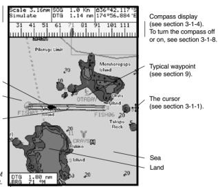
Chart is in cursor mode, press **ESC** to return to centre on boat mode (see section 3-1-1).
